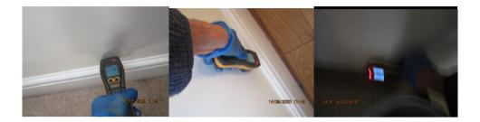
Moisture meter readings were taken throughout and evidence of high moisture content was noted particularly around the outer utility room and the main front reception rooms.
